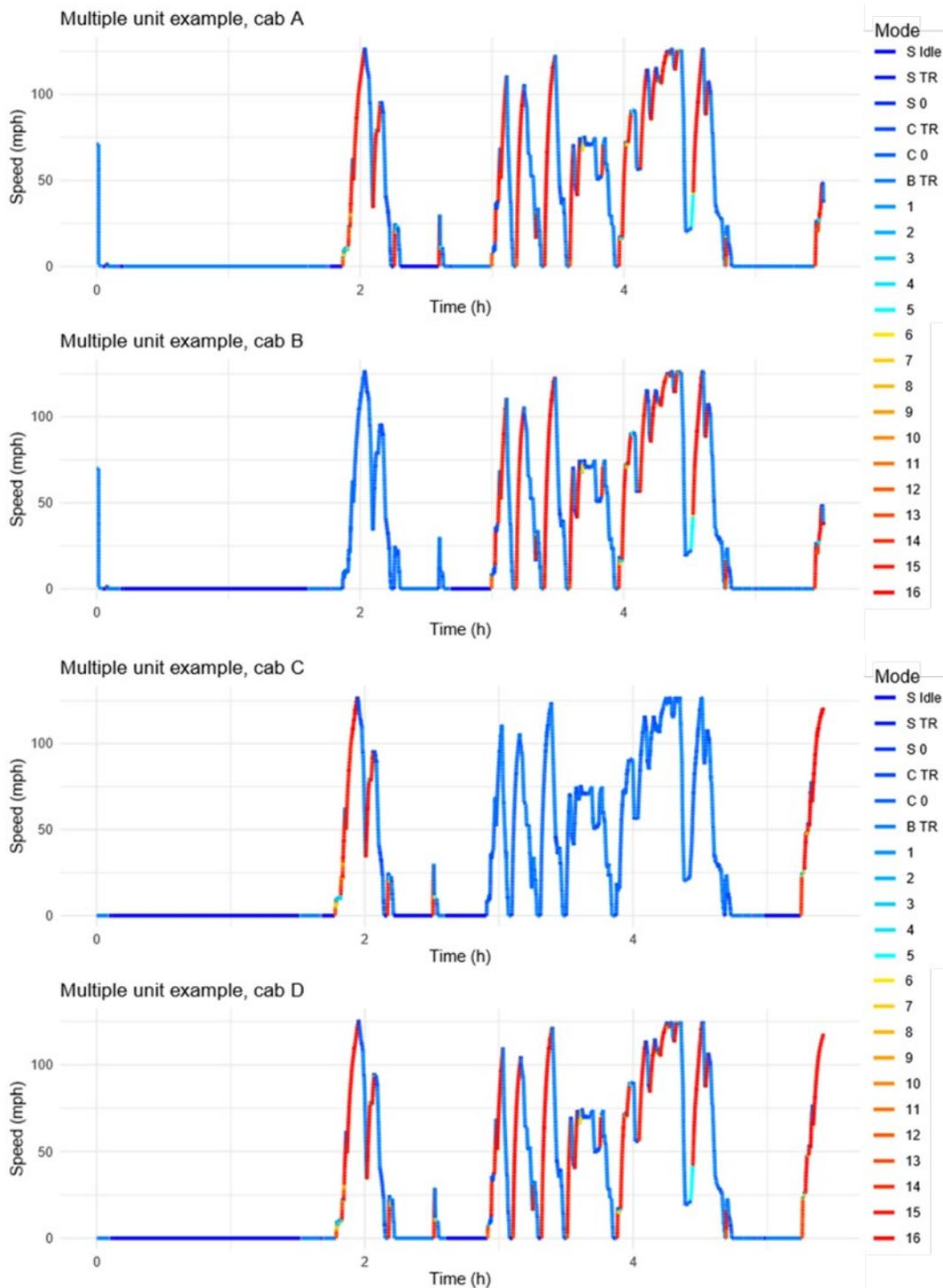
Interestingly, in the example running in multiple (Figure 22), one of the engines (cab B) was isolated for the early part of the journey before being restarted.
