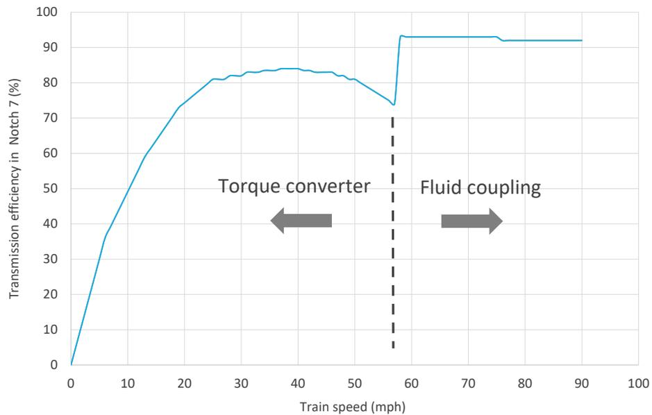
The variation in transmission efficiency with speed for trains with diesel hydraulic and diesel mechanical transmissions creates a significantly wider range of total possible emissions for Notches 1-7. The variation in emissions by engine notch (in units of g/hr) for Class 158 and 170 based on a large dataset of actual OTMR data can be seen in the boxplots<sup>13</sup> in Figure 15.
