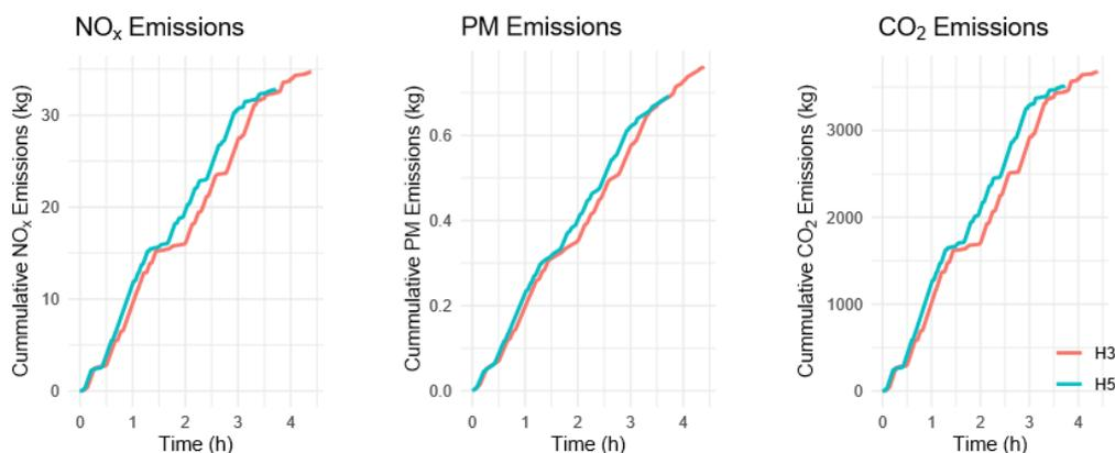
There is a section of the journey around 1.5 hours where H3 has to slow and come to a complete stop, whereas H5 slows but not for as long and does not come to a stop. This section appears to account for the majority of the differences in emissions. This particular location, where the freight train has to cross a busy mainline on the flat, is prone to congestion.
