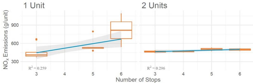
Figure 52 shows the total journey NO<sub>x</sub> emissions by number of stops. As expected, emissions for units running in multiple are higher than individual units, however as demonstrated in Figure 51 above the emissions do not double with doubled capacity.
