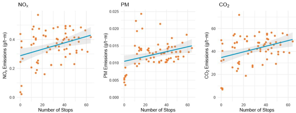
There is an increasing trend in the kg/mile emissions of each pollutant as the number of stops increases. However, the trend is not as clear as in the Class 158 and 170 passenger trains case study above. This could be due the recordings being over a range of different routes. A significant part of the difference in scale of the trend between the Class 158 and 170 and Class 220/221 is likely due to two large factors:
