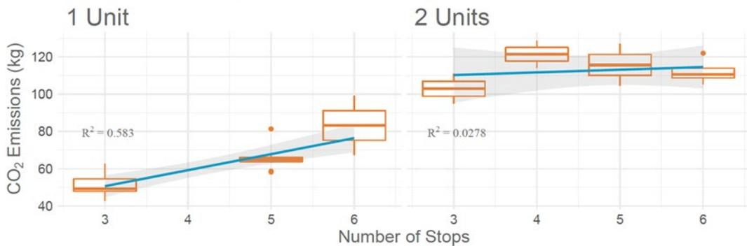
Double the capacity i.e. running two units, did not result in double the emissions. For journeys with three or five stops, total emissions of NO<sub>x</sub>, PM and CO<sub>2</sub> were on average 48% greater for units running in multiple compared to individual units.
