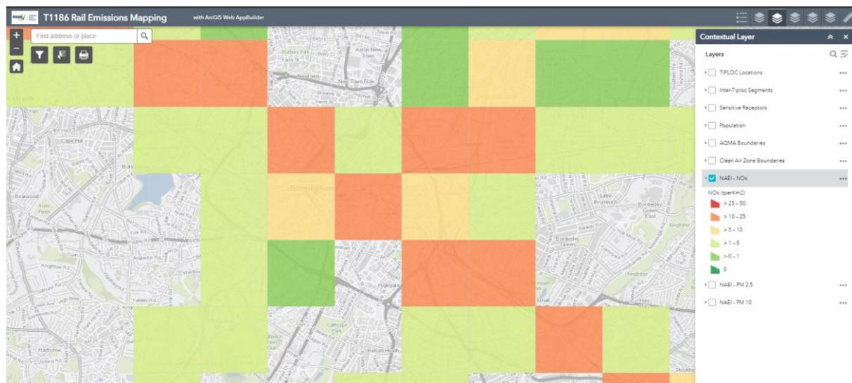
Figure 9: NAEI mapped emissions per 1 km<sup>2</sup> grid cell in the Birmingham area
