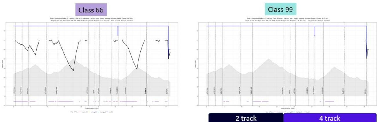
The ‘three peaks’ along this route slow down the Class 66 to over half on the line speed in places but the locomotive fairly quickly recovers on the downhill sections. The Class 99 is not slowed by the gradients at all.
