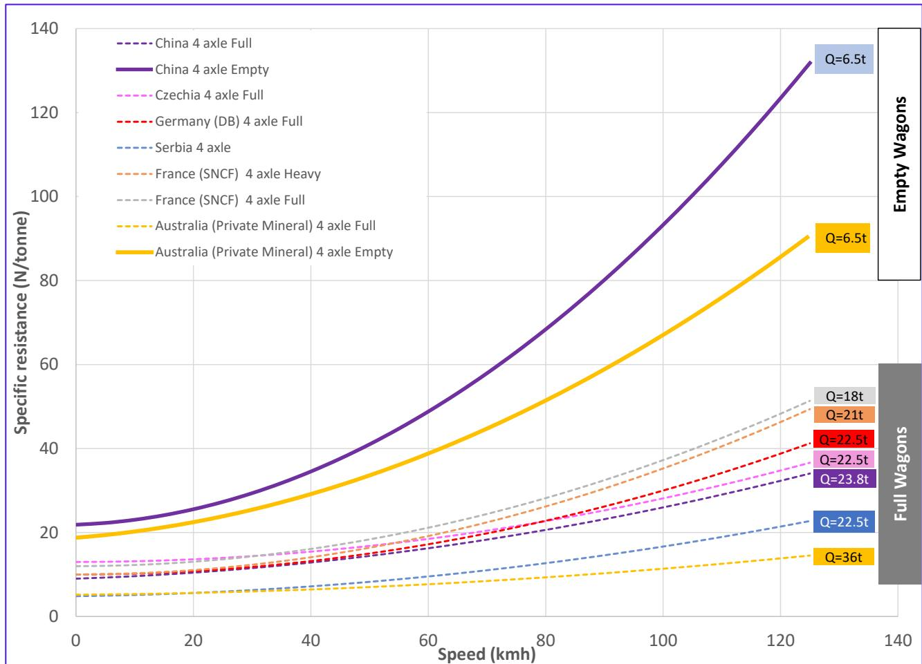
As can be seen in Figure 39 above, empty wagons (dotted lines) have much higher specific resistances than fully loaded wagons (dashed lines) and there is a reasonable range of specific resistance values between different formulae for similar axle loadings. Heavier axle loads typically lead to lower specific resistances, there are also considerable differences in specific resistance values at lower speeds between formulae which are largely a function of bearing resistance assumptions.
