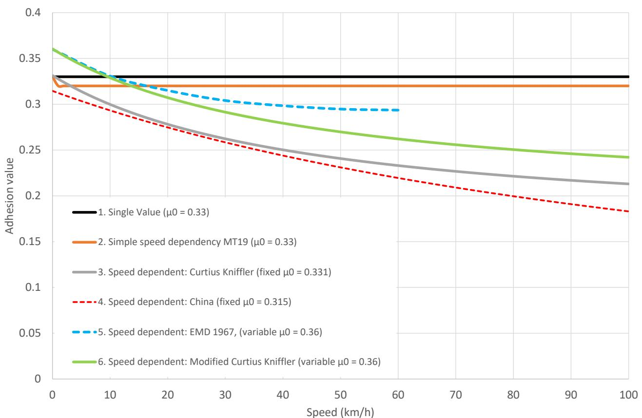
The Curtius-Kniffler curve will work at all speeds, whereas the simpler EMD curve is only valid up to 30 mph (50 km/h). Furthermore, while the EMD curve is adequate for use with diesel locomotives, it is not suitable for modern electric locomotives which can have very high tractive effort and very high deliverable adhesion above 30 mph.
