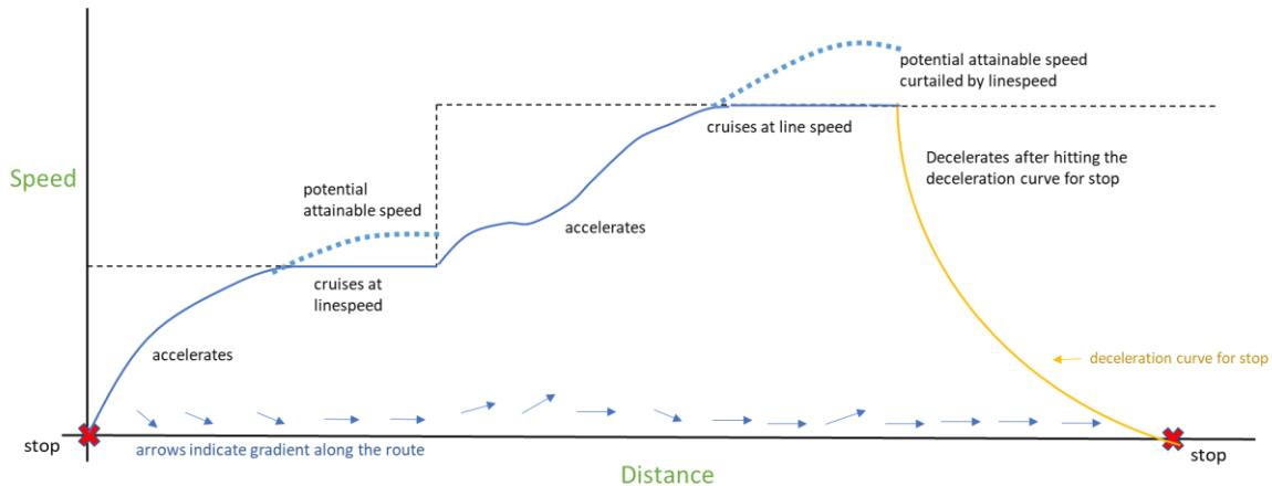
SRTcalc uses a set of modules to model the forces and dynamics of a train moving along a track. The primary focus is on calculating the force balance for each 10 m segment of track, utilising the Davis equation to calculate the net force acting on the train and the resulting acceleration, speed, and the time taken to traverse each 10 m segment of track.
