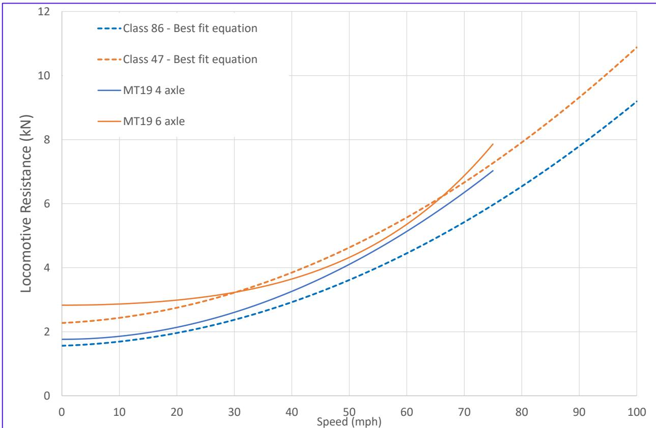
Use of the BR Class 86 (4 axles) and Class 47 (6 axles) data is recommended for default locomotive resistances where other data are not available. Use of the  $V^2 + V + \text{constant}$  equation format allows OEM data for newer locomotive types to replace the default values. Data sets are available for single and double-headed locomotive use.
