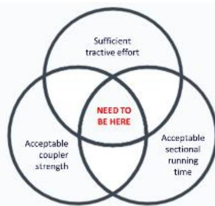
The train needs to have sufficient TE, to have an acceptable coupler strength, and to be able to progress through the network within the SRT time envelope available.
