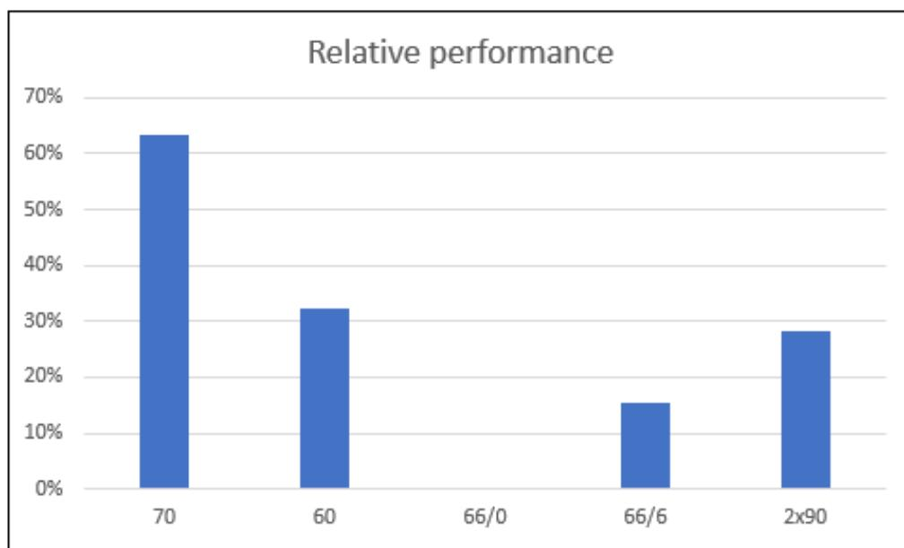
These figures should be treated with some care due to the small sample size, but the figure does show the performance advantages of all the chosen locomotive types relative to the Class 66/0s. Whilst this will be of no surprise to experienced professionals, this is the first analysis providing some empirical support to define their relative performance in real world use.
