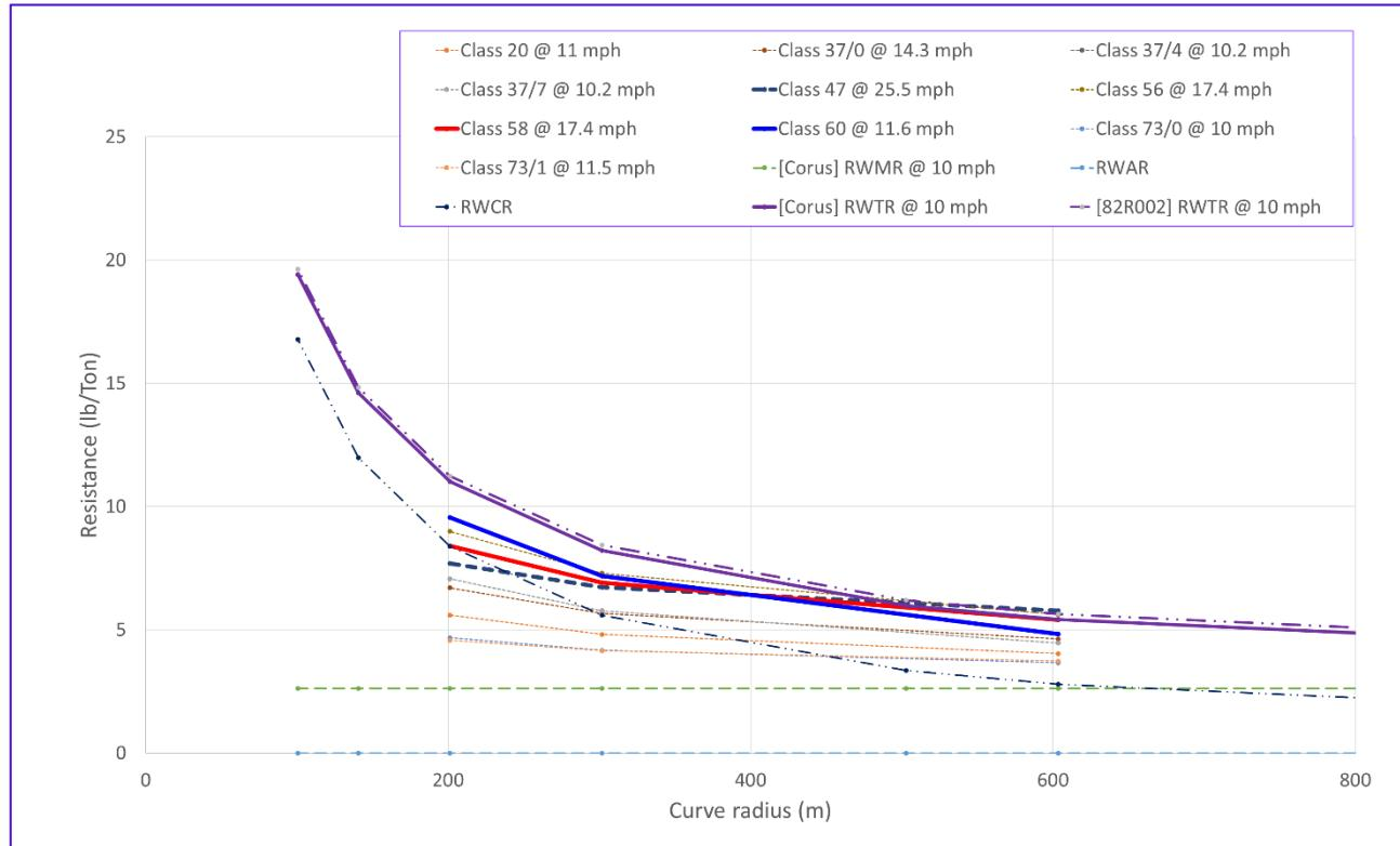
It was noted that a ‘one size fits all’ method could never match MT19 due to the large variation in wagon rolling resistance used in MT19 (as shown by the variation in wagon resistances for the different locomotives in Figure 24). It was postulated that this was due to the various ‘continuous speeds’ for each locomotive type (see Table 11), however, when these are plotted, there is no discernible correlation between speed and resistance; see Figure 25.
