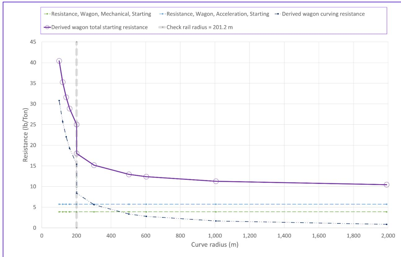
This is compared with the MT19 Table 2 and Table 4 values as shown in Figure 21. The deduced resistance is a reasonable match to the predominant values of 25, 15, and 12 lb/Ton used in MT19 (the red diamond data points in Figure 21, from Figure 9) and it sits between the higher and lower values used for the Class 73/1 and Class 60.
