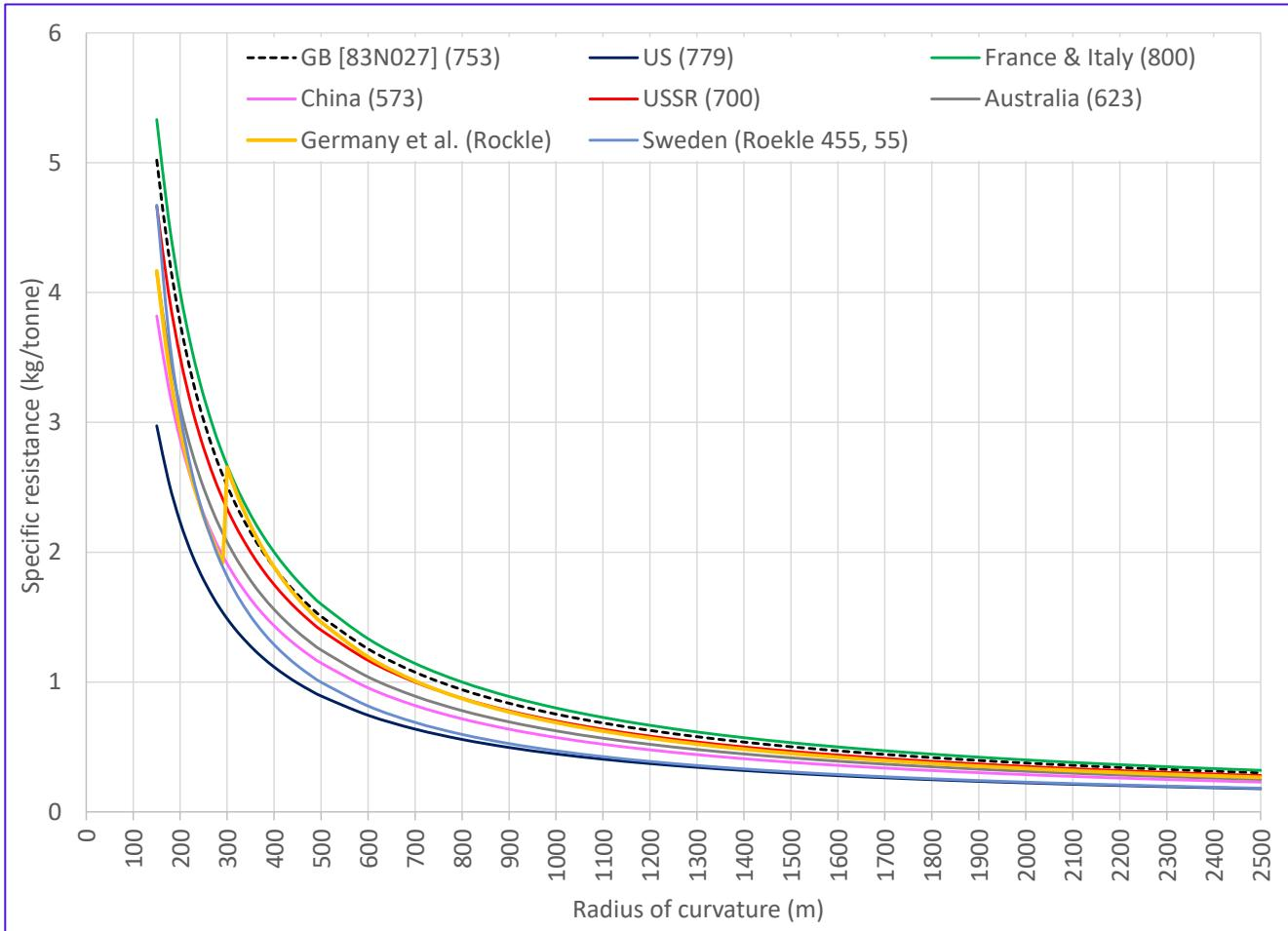
Use of the British Rail (1983) and MT19 methodology in Sections 3.3.1.2 and 3.3.2.2, that is, 753.6 kg.m/tonne (7,390 N.m/tonne), is recommended for both starting and rolling wagon curving resistance.
