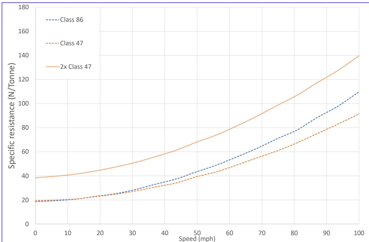
The benefit of double-heading on locomotive resistance is shown in Figure 33 where the resistance of the second locomotive is compared with the first locomotive. The resistance of the second locomotive is very similar at low speeds but falls to almost half that of the first locomotive at 100 mph.
