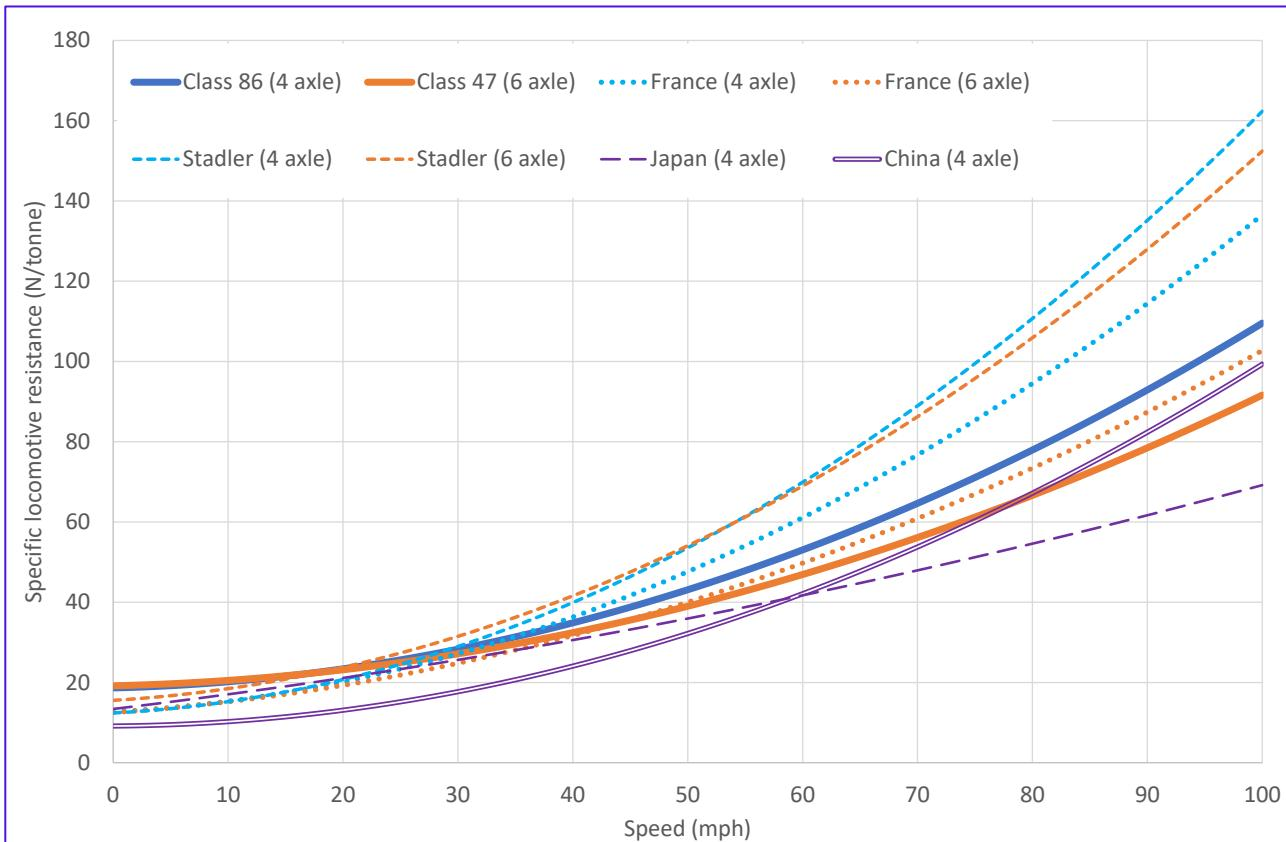
Overall mechanical resistance data from France, Japan, China, and Stadler are presented in Figure 37 below, alongside the Class 86 and 47 best-fit equations. This figure shows that the BR locomotive resistances are higher than international comparators at low speeds and similar at typically middle of the range compared against international comparators:
