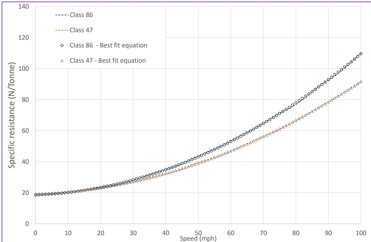
The total locomotive rolling resistances for both 4 and 6 axles using the MT19 equations and Class 86 (4 axle) and Class 47 (6 axle) are compared in Figure 35. While there are broad similarities, the variance between the two approaches for 4 and 6 axles can be up to 30%.
