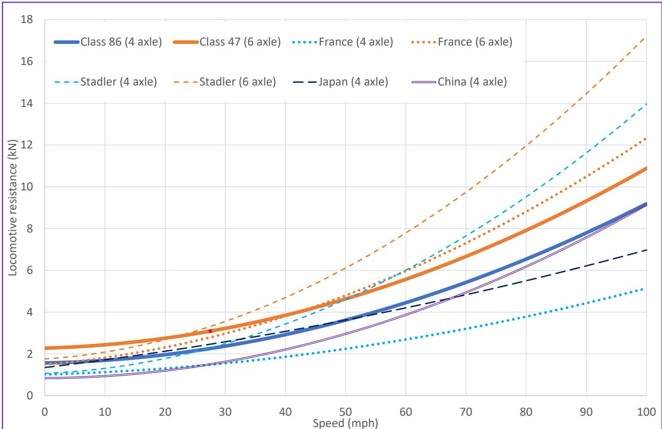
International formulae plotted in Figure 36 and Figure 37 above are presented below in standardised units of N/tonne and mph. Some formula have been adapted from the original formula but with modified coefficient values for unit conversion reasons to enable comparison between formulae. Some formulae are best-fit equations based on published curves (where formulae for those curves have not been published).
