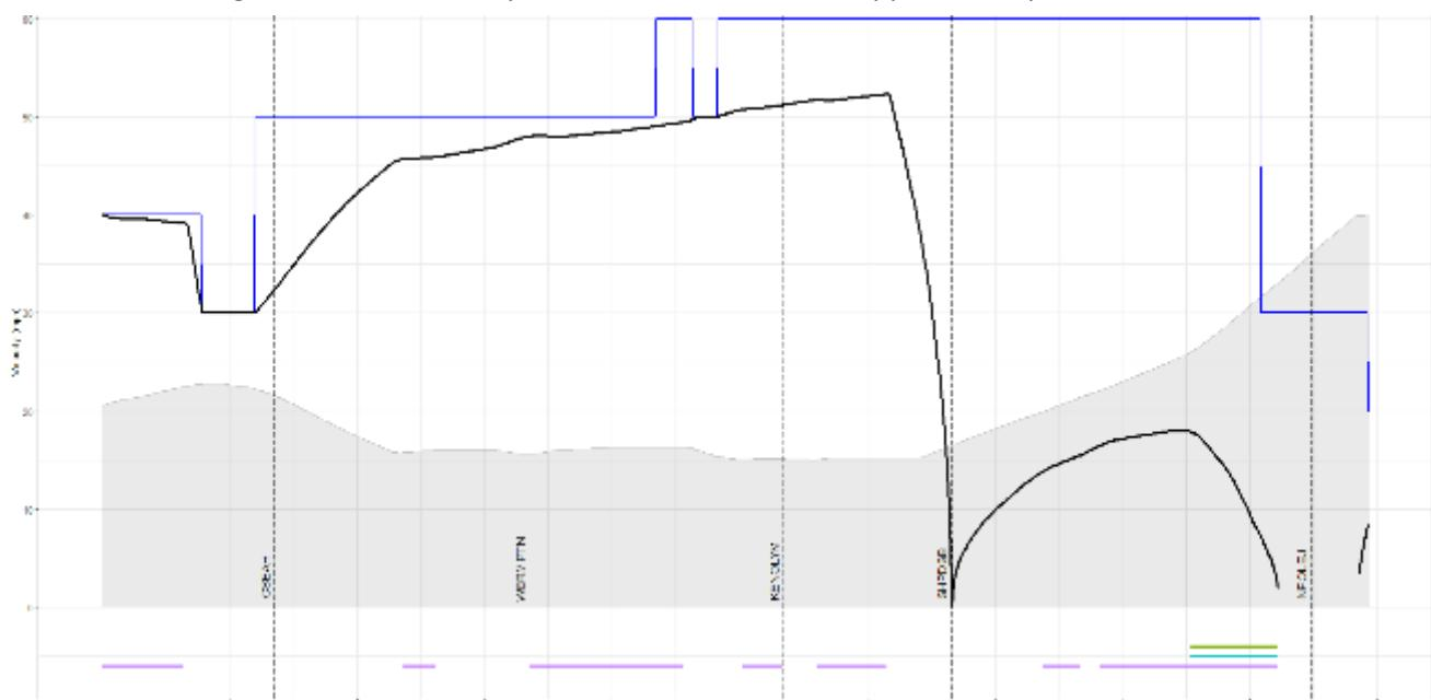
The lack of available power and momentum means that whilst the train accelerates in the initial part of the gradient but as it steepens the train comes to a halt and is then unable to restart. Note: in ‘usual’ rail head conditions the train can start, but a longer time allowance is required.
