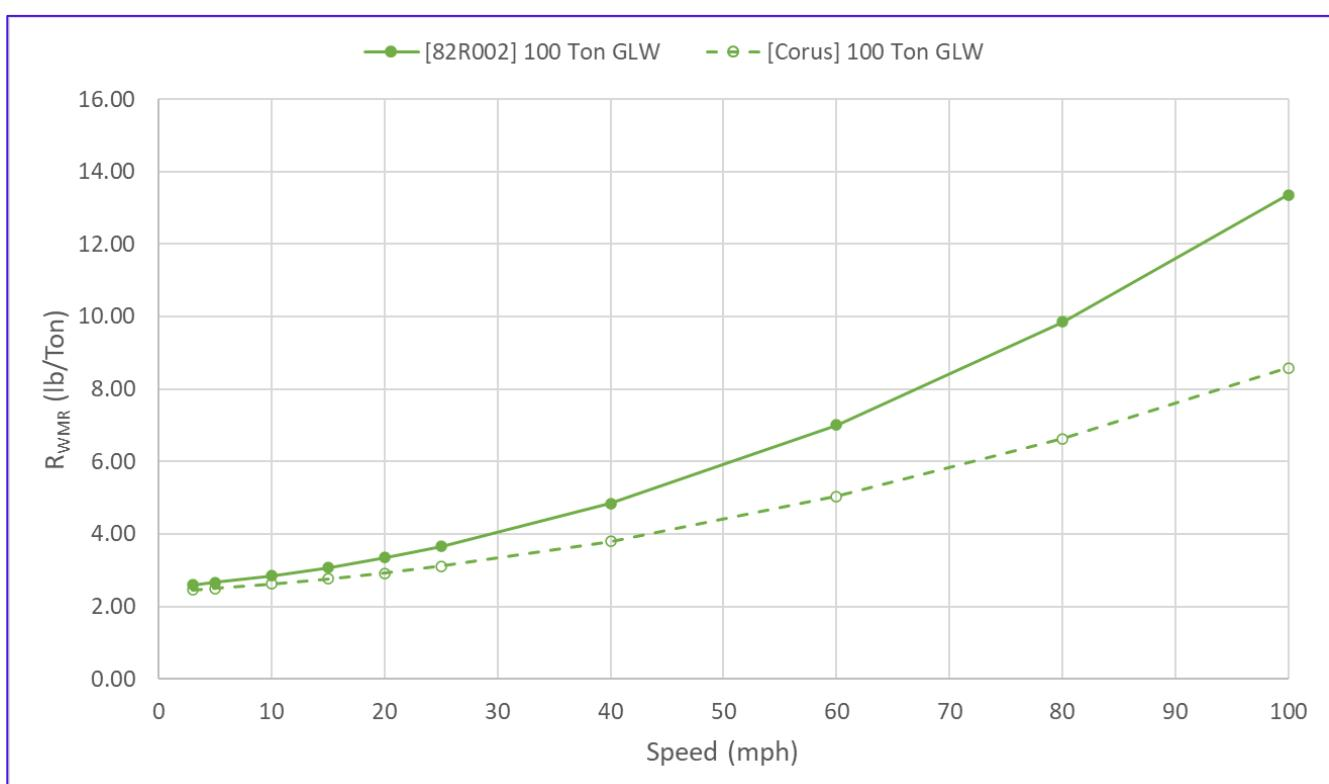
Figure 23 Resistance mechanical rolling, RWMR for various GLWs
