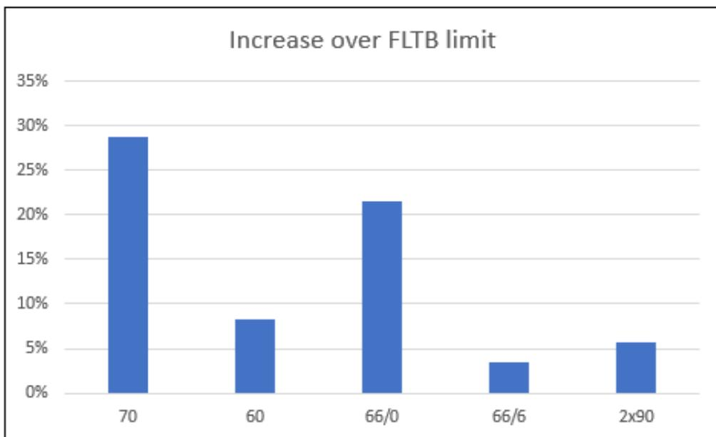
This approach sets new values where none existed for Class 70 and double headed Class 90 locomotives. The percentage increase above is over the current Class 60 limits.
