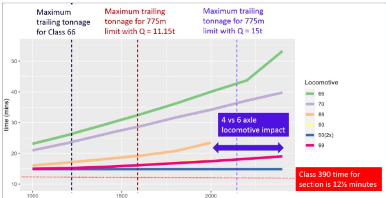
This chart shows electric locomotives are able to take significantly higher loads. As the ~25-minute SRT allowance for a Class 66 the electric locomotives can take over 2,500 tonnes, with the exception of the 4-axle Class 88 which is limited to 2,000 tonnes by its TE capability. The passenger train does not notice the gradient but is only 2.5 minutes faster than a pair of Class 90s, due to its higher maximum speed.
