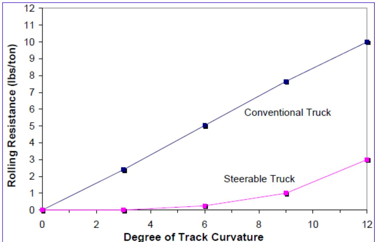
The best-fit equations below were derived for the two curves in Figure 38 based on the five available data points for each curve:
