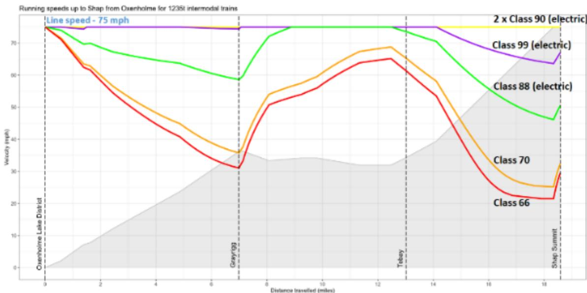
This graph clearly illustrates the benefits of electric traction which have much more TE at higher speeds than diesel locomotives. Neither the Class 66 nor Class 70 is doing 25 mph at the top of Shap on this relative light train, yet a pair of Class 90s modelled at 75 mph and the new Class 99 is modelled at around 60 mph.
