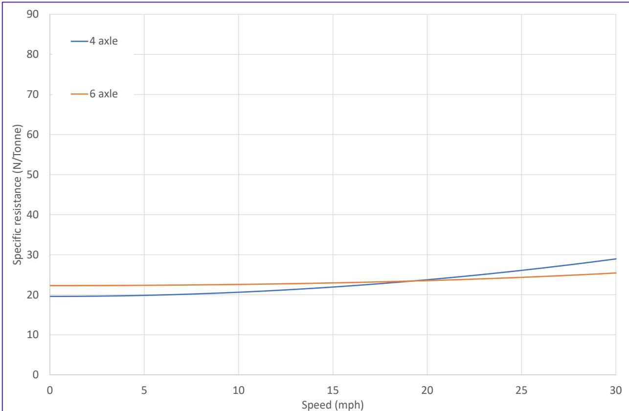
However, when the chart in Figure 29 is extended to higher speeds there is a significant divergence between the 4-axle and 6-axle locomotive specific rolling resistance curves at the higher speeds (see Figure 30).
