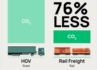
A diesel-hauled rail freight service reduces carbon emissions by 76% per tonne compared to road.
